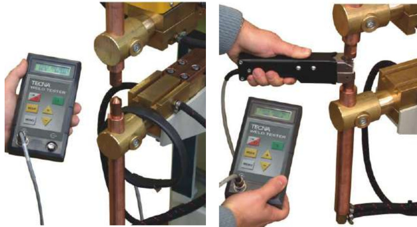
Figure 9. Rogowski coil measurement during RSW
